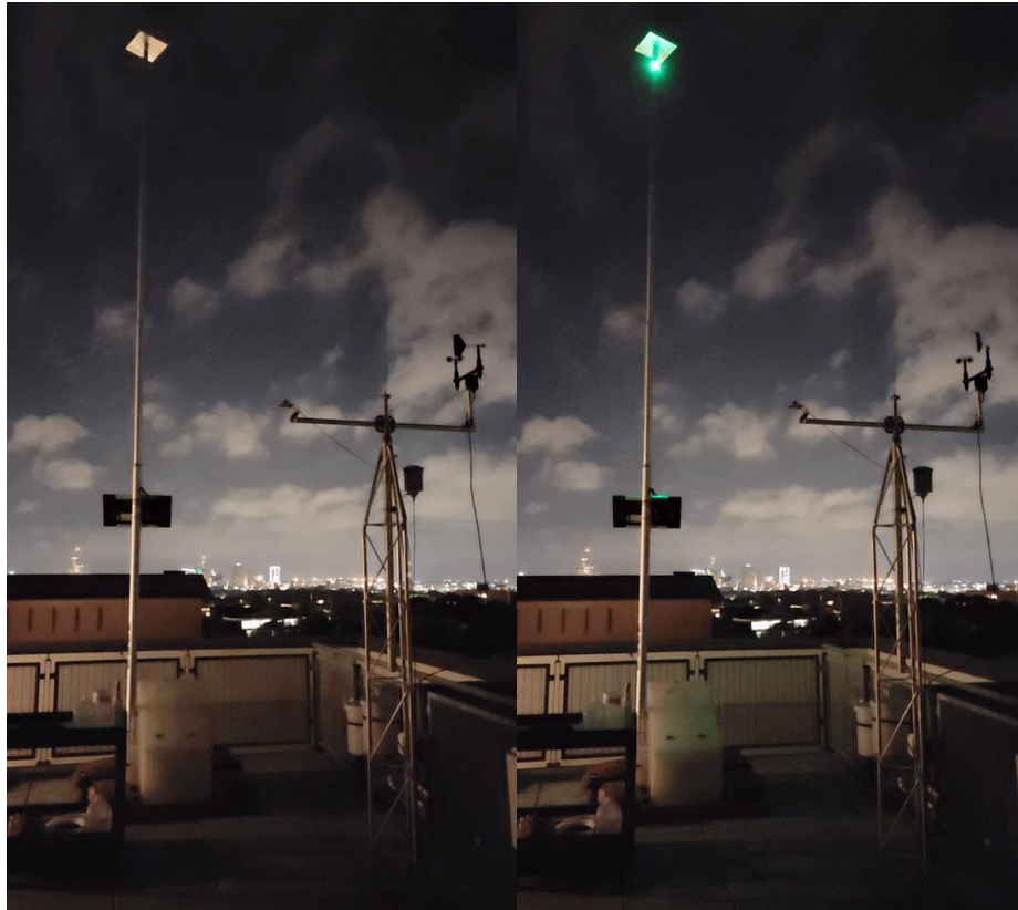
Figure 2. View of the Signal LED Flashing at Night
