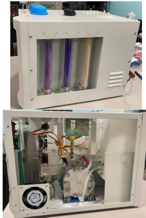
Figure 7. Side View of Hydrogen Generator (top) and Internal View of the Electrolyzer Compartment in Hydrogen Generator (bottom)
