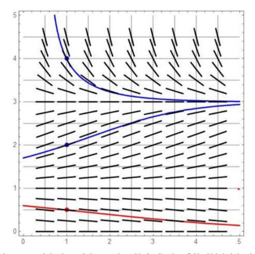
And we have presented the three solutions together with the directions field which includes the constant solutions that are dashed.
