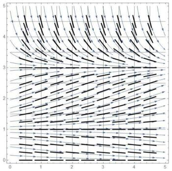
Therefore, beyond the three constant solutions, for initial conditions between 0 and 1, for the long term, the population will approach y = 0, which is a stable solution. The solution y = 1 is unstable. For initial conditions between 1 and 3 or 3 and 5, the population in the long term will approach the stable solution y = 3, from below and above, respectively. This view is also a guide for those who intend to work with the algebraic solution given by Out[16], that we write as:
