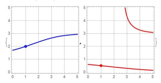
We can see that in the interval we are working for y only one level set of g corresponds to y2, but the level set corresponding to y3 also includes another solution. Therefore, we redefine the drawings to y1 and y3 in such a way that we have only the solutions we want.
