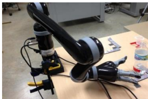
Fig. 1 Robotic arm system mounted to a table or a powered wheelchair [12].
