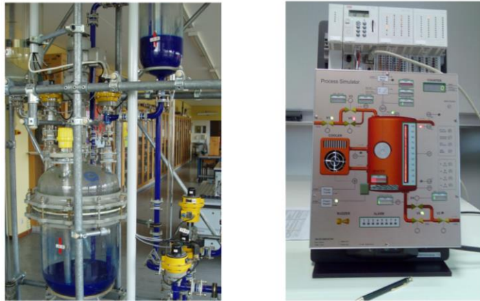
Figure 2. Pilot Plant of a Chemical Process (on the left) und hardware-model of a batch-reactor
