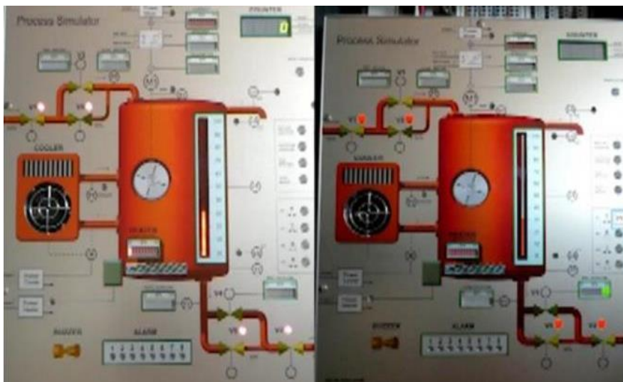
Figure 9. Digital Twin (l.), simulated and controlled with MATLAB®/Simulink. The hardware-model OSLO-3 (r.), controlled with PLC Freelance and field controller AC-700 of ABB.
