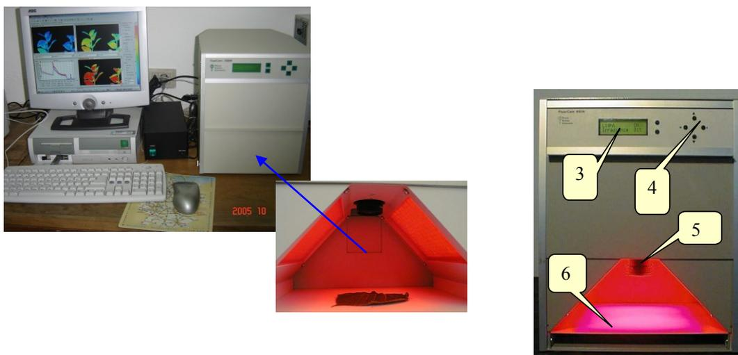
Figure 4. FluorCam System and Sample Radiation Chamber. Control panel with LCD display (3), control buttons (4), sample room with CCD camera (5) and the part where the sample is placed (6).
