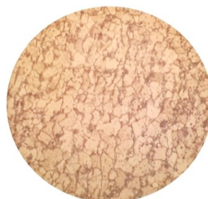
Figure 10. Micrograph for Carbon Steel which was Heat Treatment with Annealing X: 160
