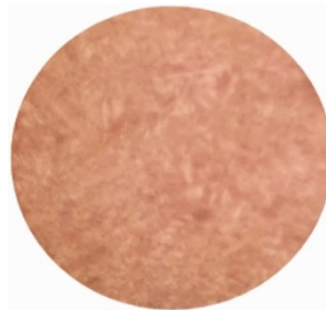
Figure 8. Micrograph for Carbon Steel which was Heat Treatment with Hardening X: 160
