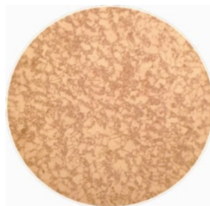
Figure 9. Micrograph for Carbon Steel which was Heat Treatment with Normalizing X: 160
