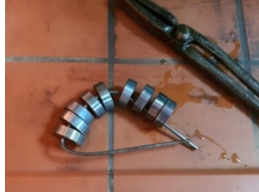
Figure 6. Normalizing Cooling Process
