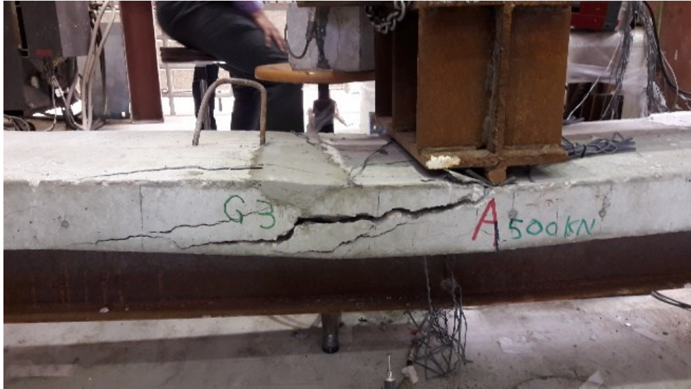
Figure 17. Shear-compression Failure at Mid-span (Experimental)
