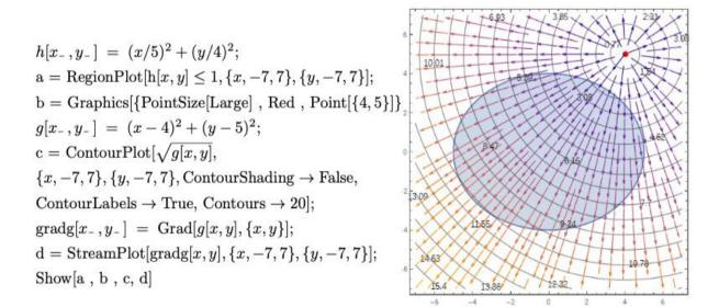
The picture shows that the shortest and the longest distances occur between boundary points of the elliptic region and the fixed point  $\{4,5\}$ . We can obtain these points by using Lagrange equations, which assert the tangency as a proportionality between gradients.
